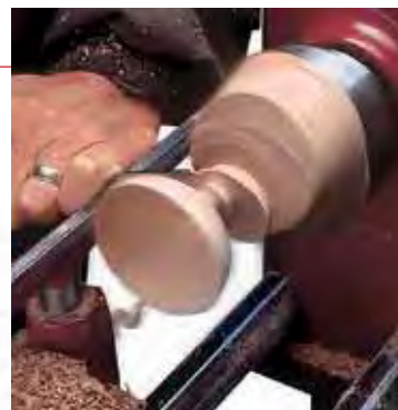
Turning a goblet with off-set stem using 0, 10 and 20mm settings.
