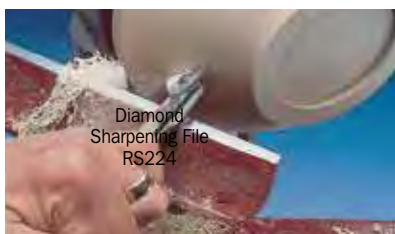
Use the straight edge for external work
