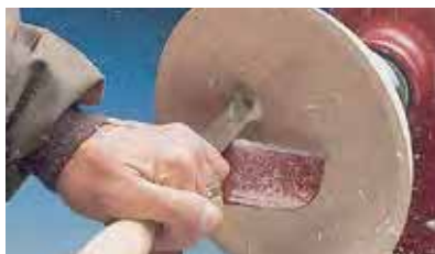
Use the curved edge for internal work
