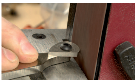
Using the woodworking chisel jig to sharpen a parting tool
