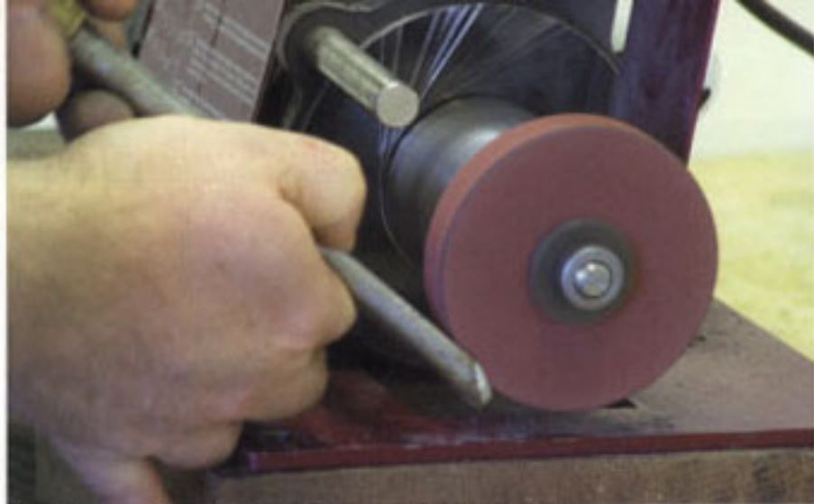
Honing the flute of a gouge using the accessory honing wheel
