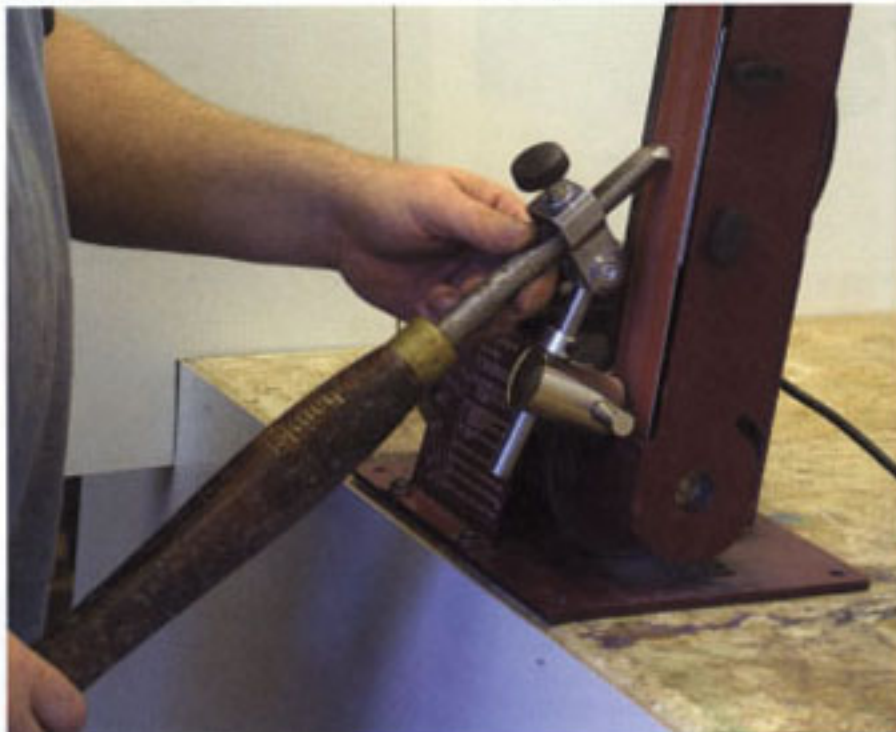
Using the fingernail profiler to sharpen a bowl gouge
