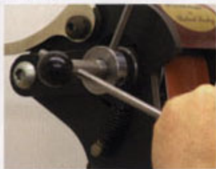
Adjusting the belt alignment
